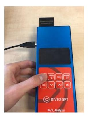
11. Once the analyzer is in the Bootloader mode (screen will remain blank) and the ON/OFF is continually pressed you will select in FLIP program RS232 window > Connect . The RS232 window will collapse. Continue to hold ON/OFF button.
